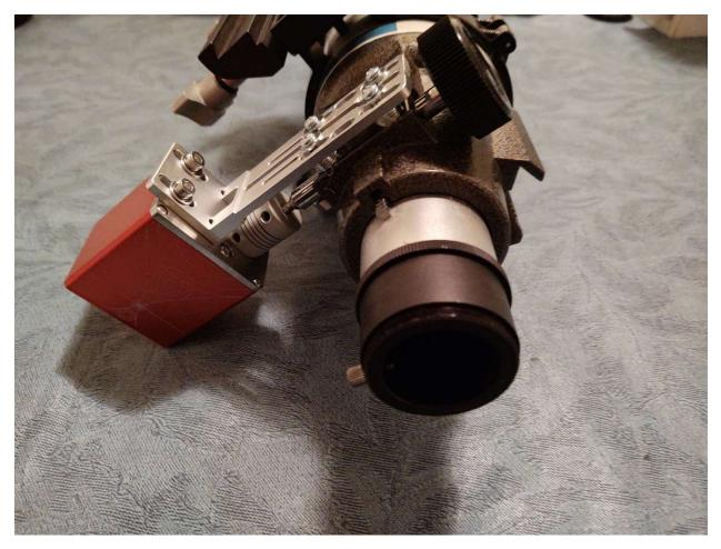
So everything is now connected and aligned. The EAF drives the focuser very smoothly. I suspect you could do the same thing on an Orion ST120 and other similar scopes.
