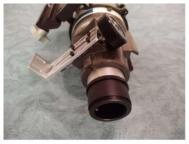
So I placed five M4 flat washers between the bracket and focuser.
