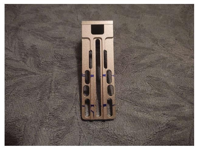
Using the cutting disk on my Dremel Tool, I cut four slots for the screws.
