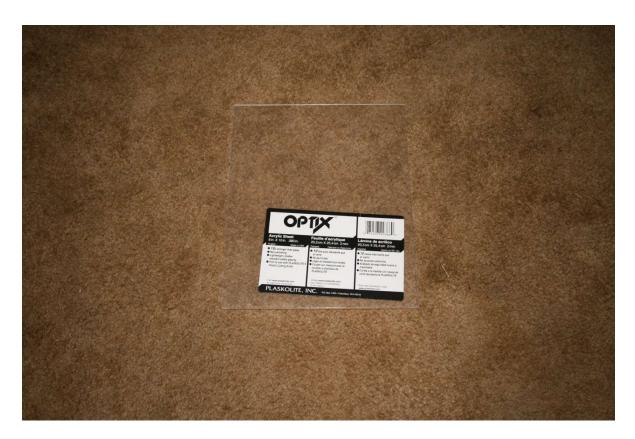
In the plastic sheet mark a circle the size of the inside diameter of your OTA. For large scopes like DOB's and SCT's you can limit this to some place between 4-6 inches. Make a second circle approximately 3/4 of an inch outside the first circle, keeping it centered over the first circle.
