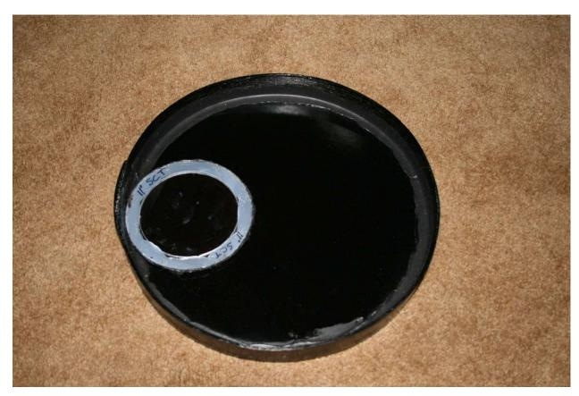
The solar filter should slide over the end of your OTA. If it doesn't stay on you could glue some felt on the inside of the wood so it fits snuggly.
