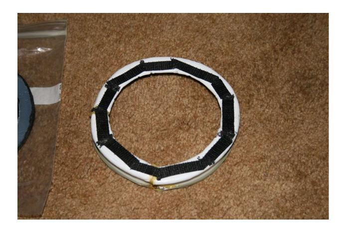
Take your black permanent marker and darken the outside of your ring and any silicone to prevent light leaks. Put your mounting ring over the end of the OTA and put the filter over the end of the mounting ring.
