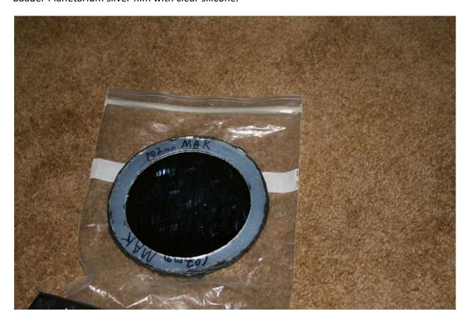
Make a circle out of something that will fit snuggly over the end of the OTA, that you can use as a mounting ring. I used some foam filled vinyl flexible storm door weather strip and reformed it to a curve using a heat gun. You could probably use a hair dryer too. Glue the ends together and let it dry. Cover one side of the filter rings with Velcro. Put the other side of the Velcro on the outside of the mounting ring. Be sure and have the the Velcro ends met up so no light leaks in.
